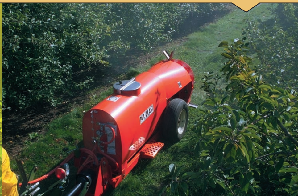
200 gallon tank, narrow profile, modular tongue, 28" fixed pitch fan, A/R 904 pump.
