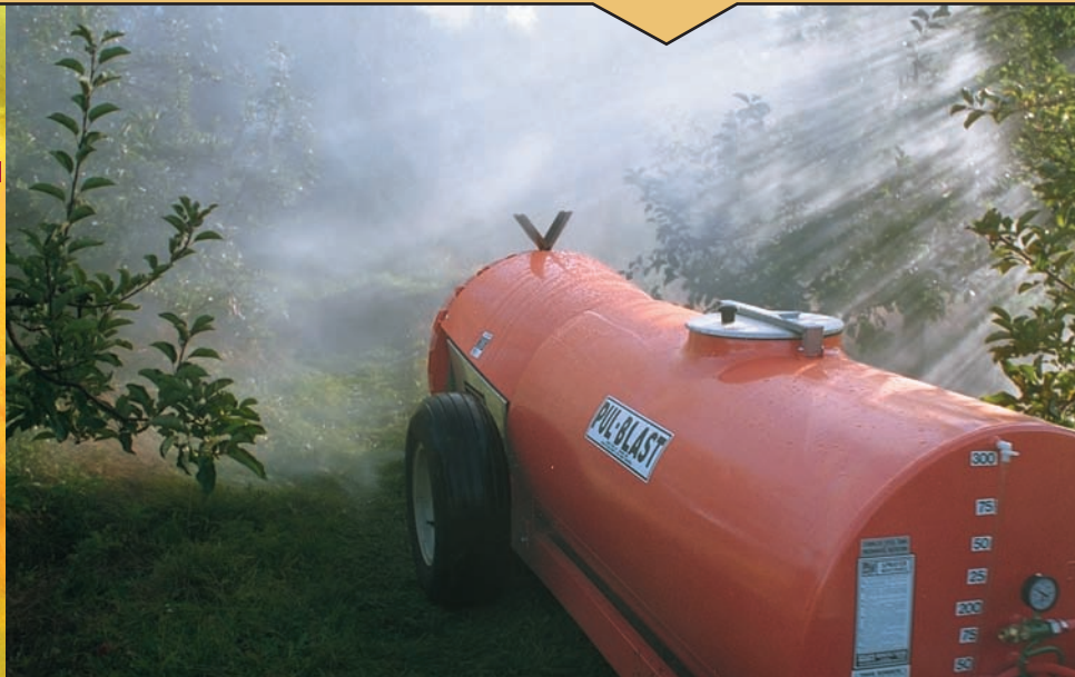
200 gallon tank, narrow profile, modular tongue, 28" fixed pitch fan, A/R 904 pump.
