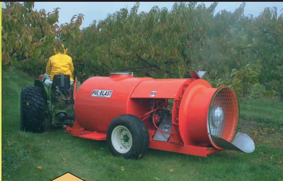
300 gallon tank, standard profile, 32" variable pitch fan, A/R 150 pump.
