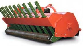
SPF with rakes installed. Rakes float to trace terrain contours.
